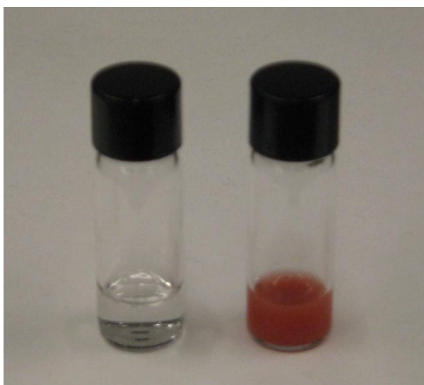
Figure 7.24: ZnSe quantum dots coated in lipid-PEG, prepared fresh (left) and after sitting at room temperature for 4 months (right).
